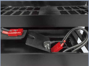
Battery side roll out and built-in charger are standard features of the stock picker. This allows for easy battery replacement and convenient charging.
