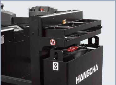
The rear load tray can be folded to allow for working in a confined space.
